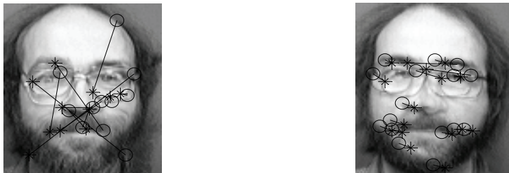
(c) Both images overlaid and RANSAC robust F estimation on matched feature points
